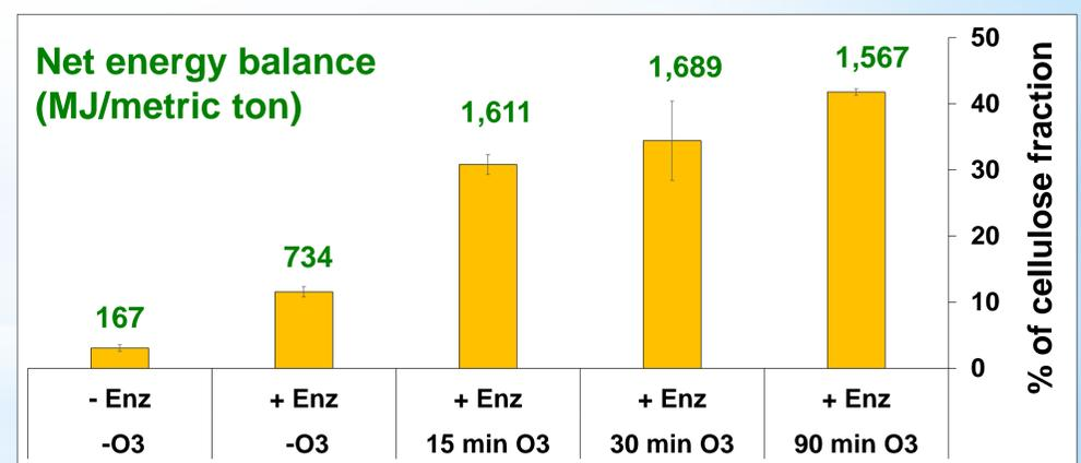
Figure 8: Sugar release after ozonation followed 72 hr Saccharification (black) showing that reducing 75% of ozonation time (15 min instead of 90 min) yielded in 25% less sugar conversion (30% instead of 40%). The net energy balance (green) is showing a reduction at higher ozone dose, demonstrating increased process efficiency at lower ozone doses
