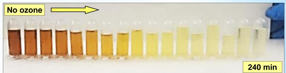
Figure 6: Changes in color waste solubles through ozonation from brown (left, untreated) till milky white (right, 240 min)
