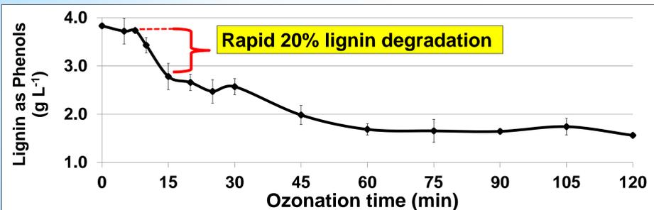
Figure 4: Lignin alkali ( $4 \text{ gL}^{-1}$ ) degradation as determined by phenol content via Folin-Ciocalteu (F-C) assay
