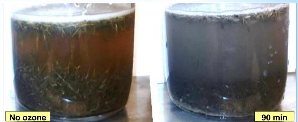
Figure 7: Before ozonation (left) and after 90 min ozonation (right)
