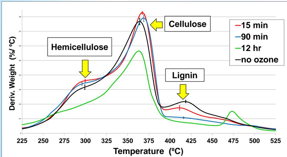
Figure 3: Thermo-Gravimetric Analysis (TGA) results showing lignin reduction accompanied with the appearance of hemicellulose. The amount of the three substances is calculated as the area ( $\int$ ) under the substances specific curve
